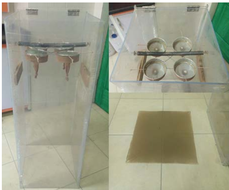
Figure 1 Soil dust chamber designed in this study to dust the plants. The rayon cloth attached at the bottom of each screen helped distribute the soil evenly.
