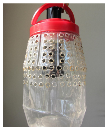
Figure 1 The blacklight trap designed for Tuta absoluta .
